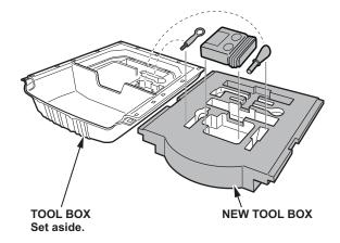
8. Install the jack, the wheel nut wrench/jack handle, and the extension bar into the new tool box.
