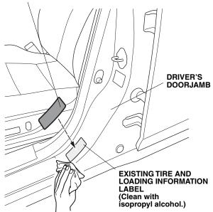
Remove the adhesive backing from the new TIRE AND LOADING INFORMATION label and apply it over the existing label.
