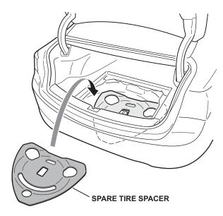
11. Install the spare tire assembly into the spare tire area (label side down), and secure it to the vehicle using the spare tire bolt provided. Tighten the bolt securely.
