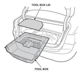
7. Transfer the tools from the old tool box to the new tool box.
